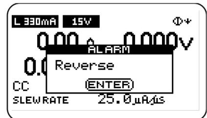
Fig. 2-12 Reverse connection alarm
