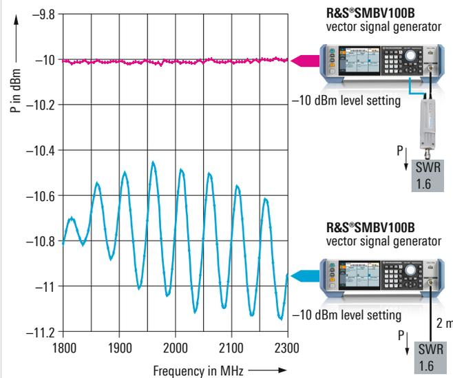
Upper graph: using the R&S®NRP-Z28, with activated user correction;
