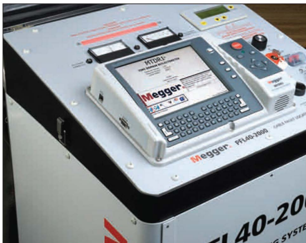
The MTDR shown mounted in the Megger PFL40A cable fault finding system
