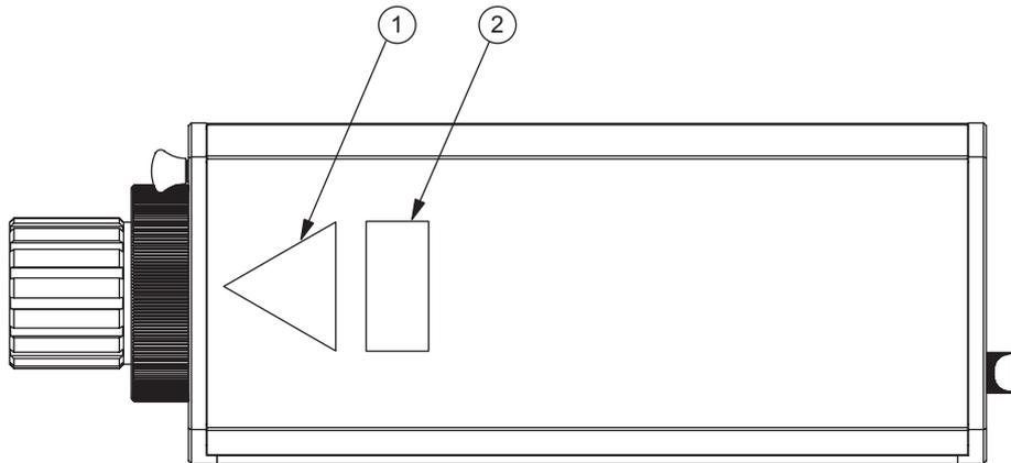
Figure 1.2: Position of the laser warning labels on the sensor head OFV-303/-353 in EC countries
