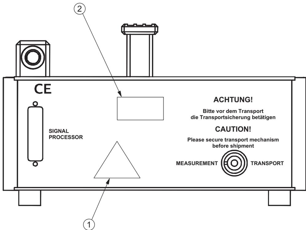
Figure 1.3: Position of the laser warning labels on the sensor head OFV-511/-512 in EC countries
