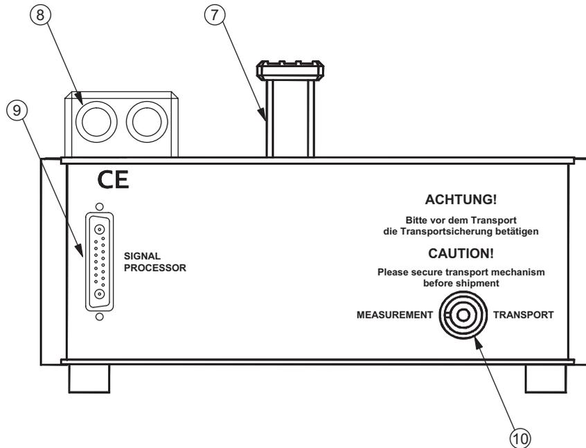
Figure 3.8: Rear view of the sensor head OFV-512
