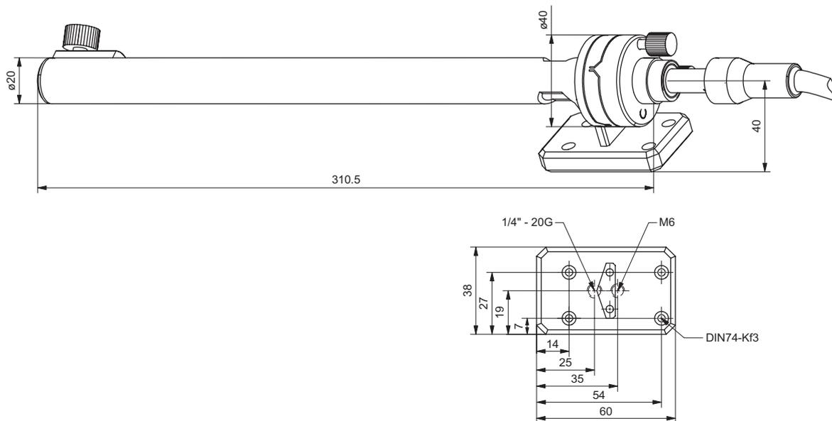
Figure B.1: Side view and bottom view of the reference head OFV-152 (dimensions not specified are given in mm)
