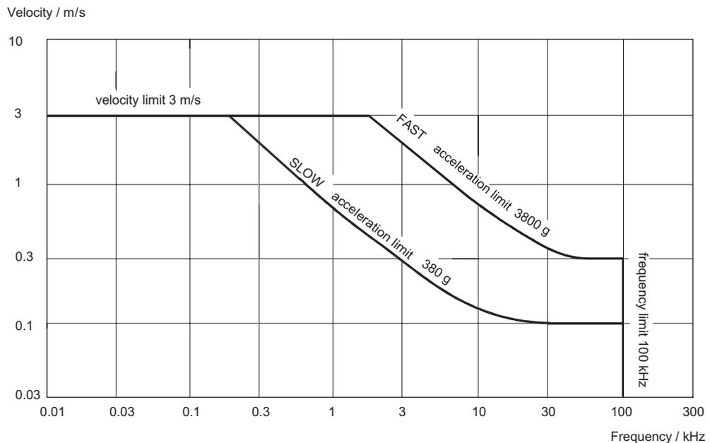
Figure 4.1: Range diagram of the tracking filter
