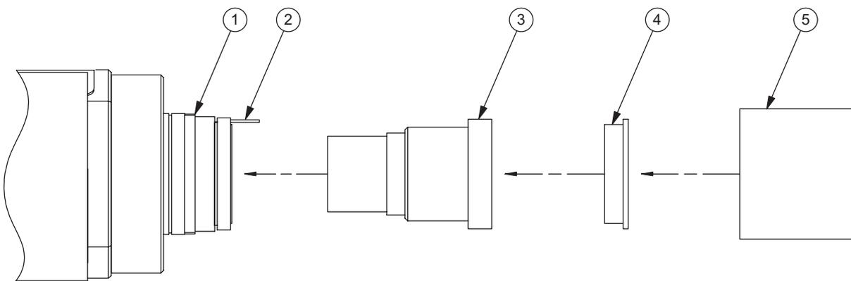
Figure 5.1: The components of the front lens mount
