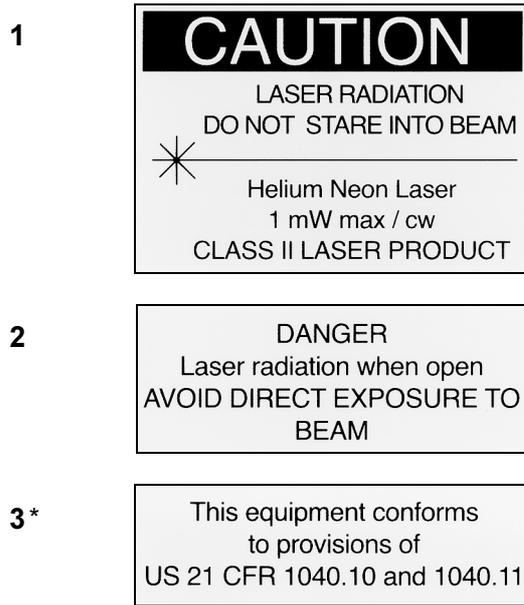
Figure 1.4: Laser warning labels for the vibrometer in non-EC countries (\*only within the USA)
