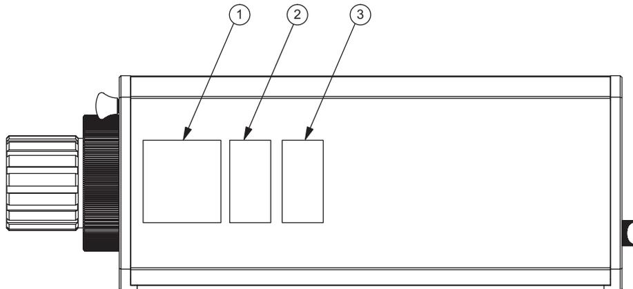
Figure 1.5: Position of the laser warning labels on the sensor head OFV-303/-353 in non-EC countries
