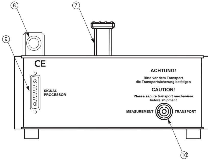
Figure 3.6: Rear view of the sensor head OFV-511
