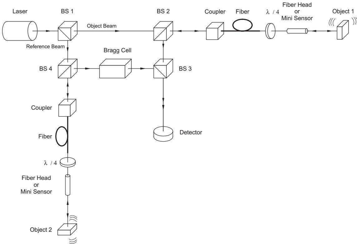
Figure C.3: Optical configuration of the interferometer in the sensor head OFV-512
