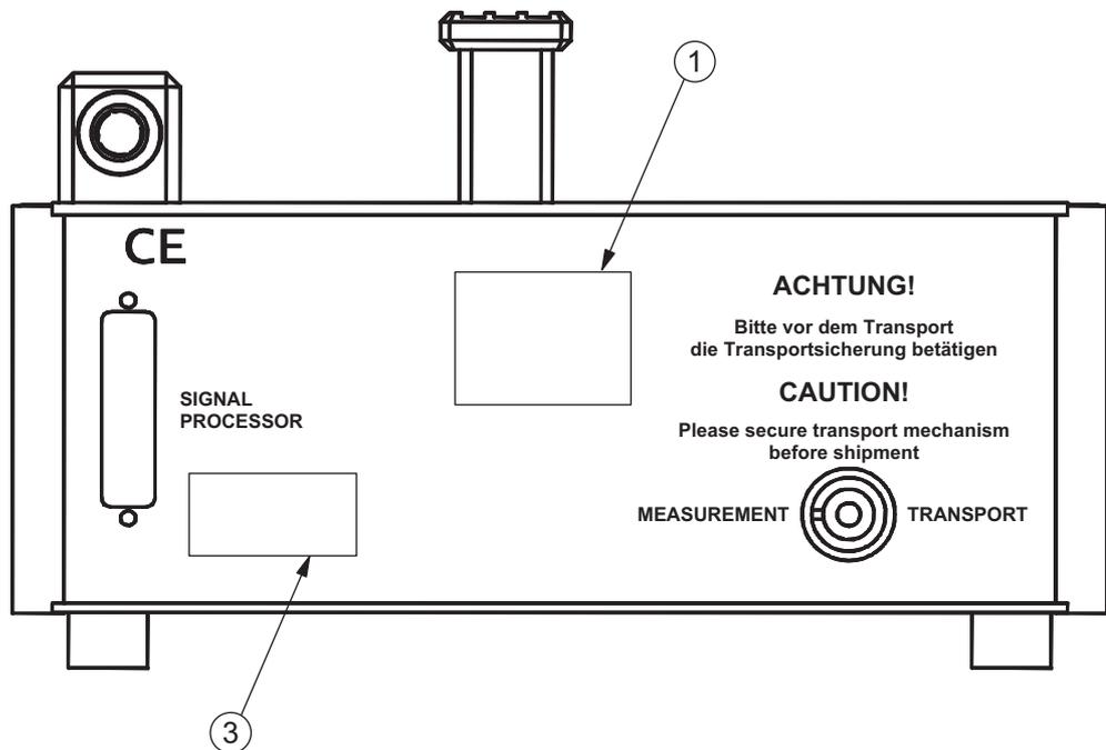
Figure 1.6: Position of the laser warning labels on the sensor head OFV-511/512 in non-EC countries
