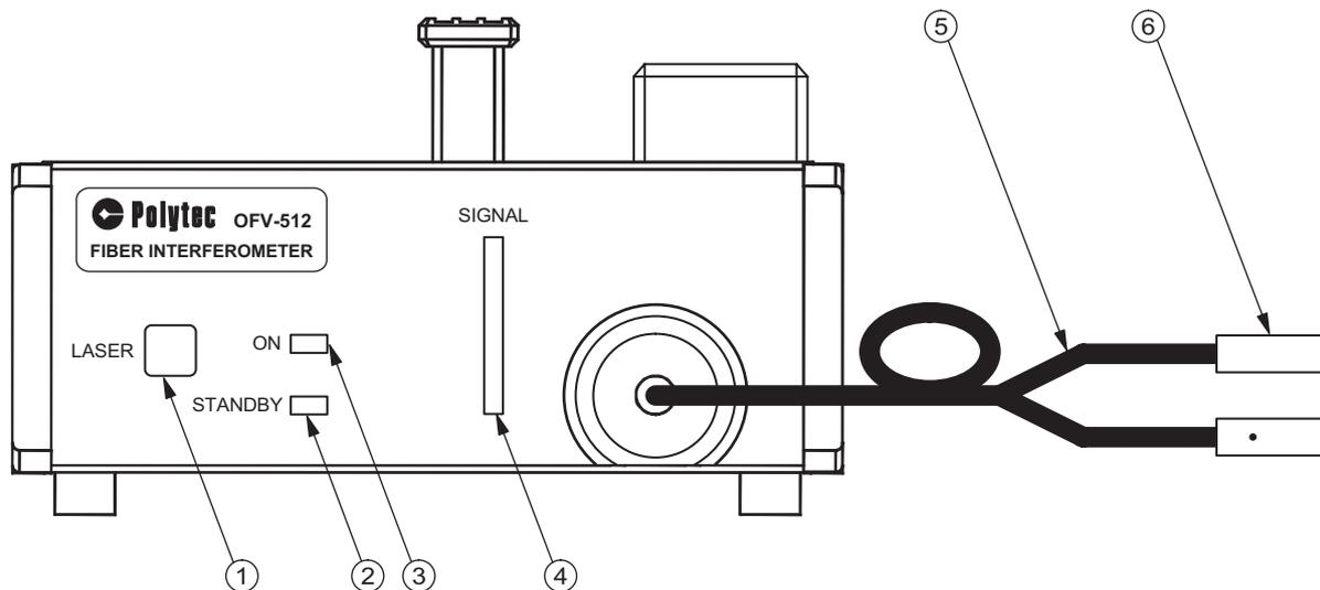
Figure 3.7: Front view of the sensor head OFV-512
