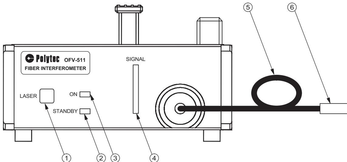
Figure 3.5: Front view of the sensor head OFV-511
