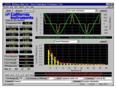
Both Voltage and Current waveforms are shown in real-time. For class A and D test, the special waveshape template (red) is shown.
