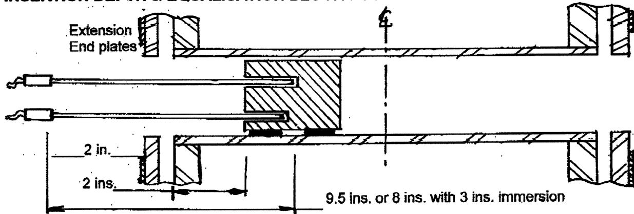
**INSERTION DEPTH & EQUALISATION BLOCK POSITION - "EXTRA SHORT" PROBES**
