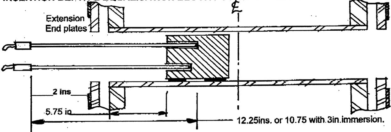
**INSERTION DEPTH & EQUALISATION BLOCK POSITION - "SHORT" PROBE LENGTHS**
