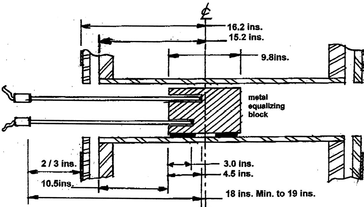
INSERTION DEPTH & EQUALIZING BLOCK POSITION -- "STANDARD" PROBES
