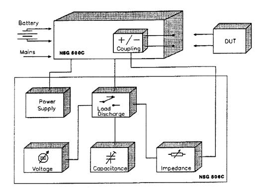
The two-part Generator, Type NSG 506C, has been designed as an auxiliary unit for the NSG 500C and enables the production of high energy pulses (pulses 5 and 7).
